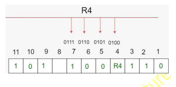
To find the redundant bit R4, we check for even parity. Since the total number of 1's in all the bit positions corresponding to R4 is odd the value of R4(parity bit's value) = 1
