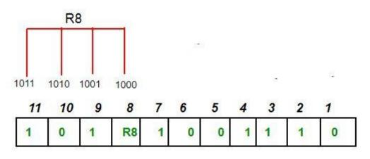
To find the redundant bit R8, we check for even parity. Since the total number of 1's in all the bit positions corresponding to R8 is an even number the value of R8(parity bit's value)=0. Thus, the data transferred is:
