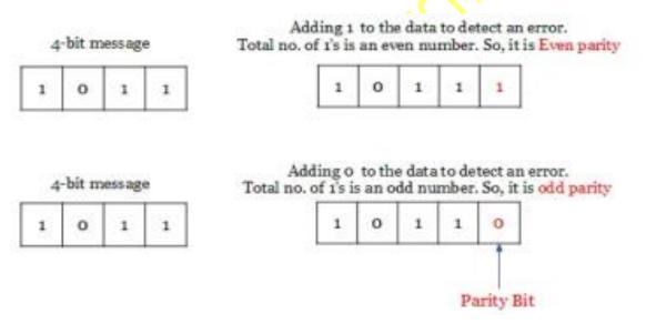
The following table shows the some of the 4-bit messages to be transmitted along with the parity bits. The bits in bold are the parity bits.
