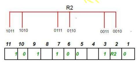
To find the redundant bit R2, we check for even parity. Since the total number of 1's in all the bit positions corresponding to R2 is odd the value of R2(parity bit's value)=1
