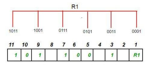
To find the redundant bit R1, we check for even parity. Since the total number of 1's in all the bit positions corresponding to R1 is an even number the value of R1 (parity bit's value) = 0
